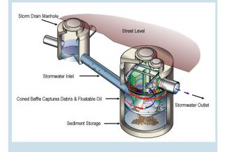
The West Union Street Improvement Project included the installation of a Manufactured Water Quality System to treat stormwater from approximately 136 acres of the west side of the City.
